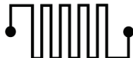
Figure I.2, Example meander structure that could be used to optimize a thin film thermistor
